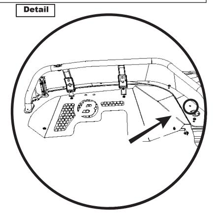
Gently push back the Fender Liner, so you can insert the Nut plate (20064138) behind the vehicle fender. Make sure to place the flate side of the Nut Plate against the fender sheetmetal. Insert M8 Allen Bolt (3000786) with Lock Washer (3000147) and Flat Washer (3000303) as shown.
