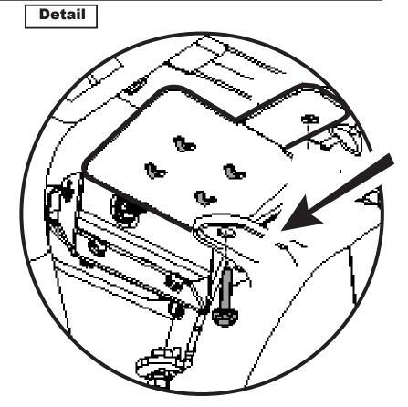
Once the Harness is secured, Install the OEM bolt into the ClipNut from the OEM plastic fender, into the Body Mount location, from the underside, as shown.
