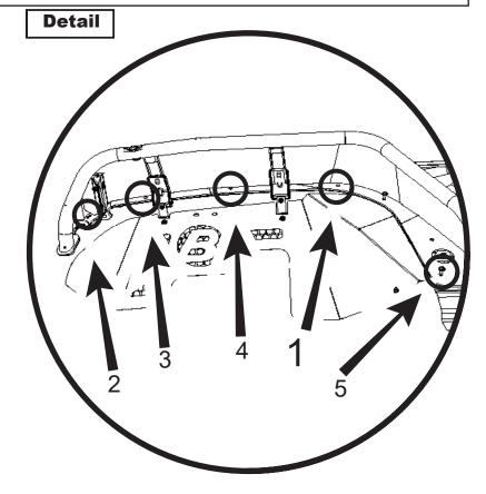
Stack-up the hardware with M6 Allen Bolt (3000742), M6 Lock washer (3000136) and M6 Flat Washer (3000288), install the M6 Flange Nut on the backside of all the components.
