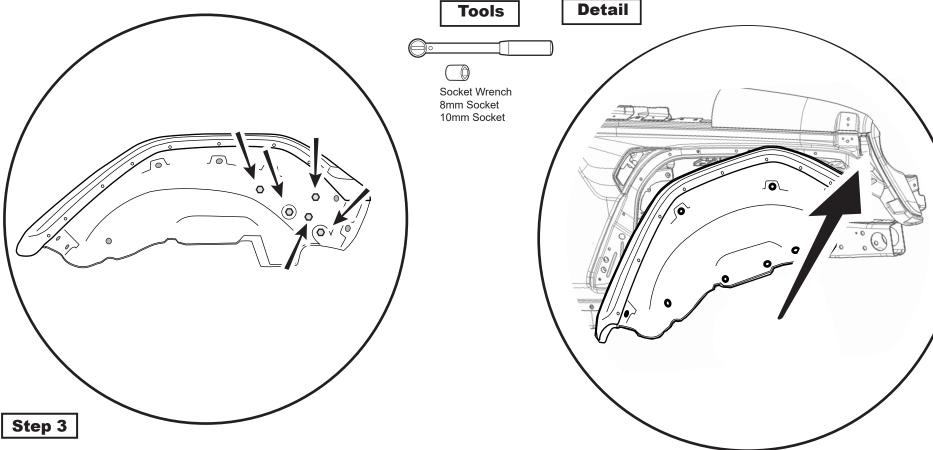
Now remove the last inner bolts that are holding the splash shield to the DRL fender light. There are five (5) bolts to remove,
