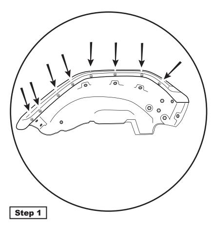
On the OEM front fenders, It may be easier to cut the head of the retainer off with Side-cutters and remove. These 8 fasteners will not be reused.
