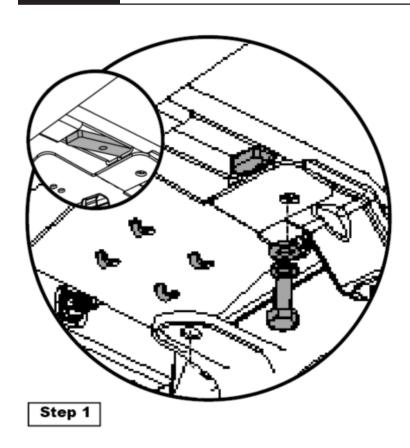
Insert the final Nut Plate (20064138) into the Fender Flare slot above the OEM fender hangers body mount. Install M8 Bolt (3002578) with M8 Lockwasher (3000147), and M8 Flatwasher (3000303) through the hole in the Harness Blocking Plate, and body mount, into the Nut Plate as shown.
