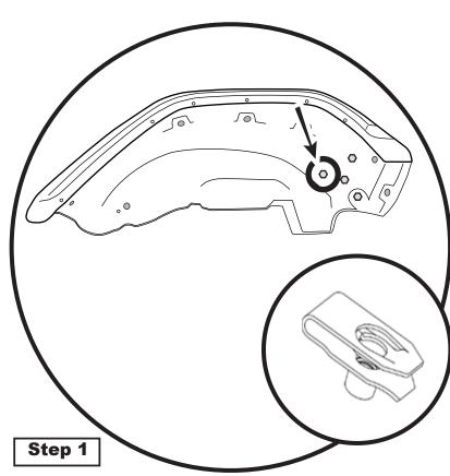
Remove the ClipNut from the OEM plastic fender, in the location shown. The OEM Flange bold will also be needed .
