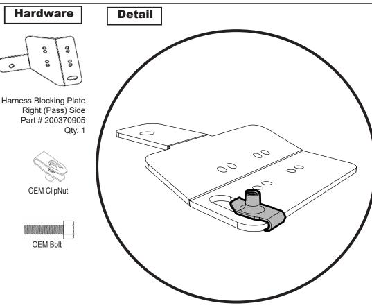
Install the ClipNut from the OEM plastic fender, onto the location shown. The OEM Flange bold will also be needed.
