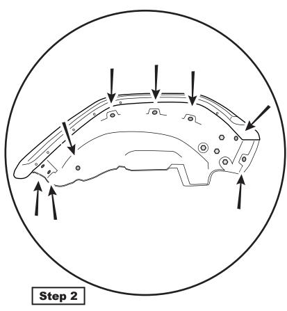
Next, releasing the inner fender liner push-in retainers. Use a Panel tool to pry all the plastic trees that join the liner to the Jeep body.
