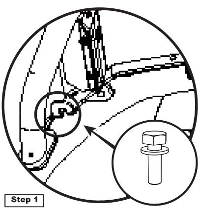
Insert M8 Bolt (3002578) and M8 Washer (3000303) from above the flange, and through the body mount as shown above.
