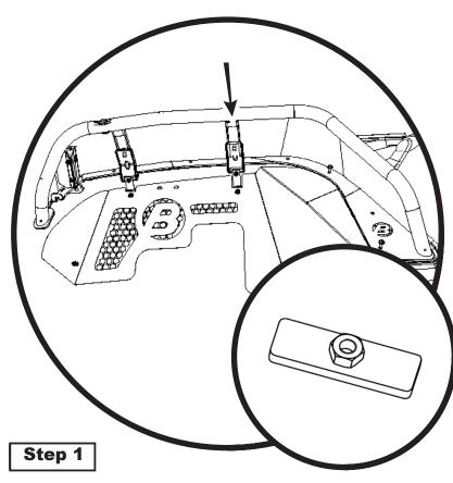
Place the Fender Flare in position onto the OEM fender hangers. Insert Nut plate (20064138) into the OEM hanger as shown. Loosely install the hardware M8 Bolt (3002578) with M8 Lockwasher (3000147), and M8 Flat-washer (3000303) as shown
